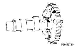
3. Measure the camshaft lobe. Replace if out of specification.
