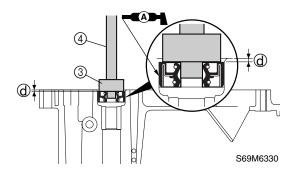
Ball bearing attachment ③: 90890-06638 Driver rod LS ④: 90890-06606
