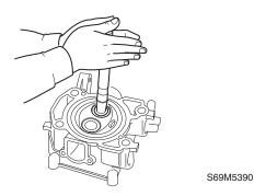
4. Measure the valve seat contact width ⓐ where the blueing dye is adhered to the valve face. Reface the valve seat if the valve is not seated properly or if the valve seat contact width is out of specification. Replace the valve guide if the valve seat contact is uneven.
