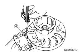
4. Tighten the bolts, and then check the TCI unit air gap. Adjust if necessary.
