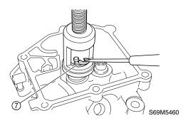
4. Lightly tap the valve spring retainer with a plastic hammer to set the valve cotter securely.
