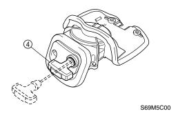
9. Install the choke knob assembly.
