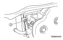
6. After adjusting the engine idle speed, adjust the throttle cable.
