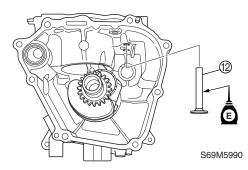
8. Set the camshaft (3) into the cylinder block as shown.
