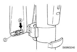
Place a drain pan under the drain screw
