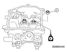
2. Install the valve ②, valve spring ③, and valve spring retainer ④ in the sequence shown, and then attach the special service tool.
