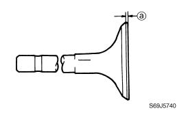
Valve margin thickness (a): Intake: 0.7 mm (0.028 in) Exhaust: 1.0 mm (0.040 in)
