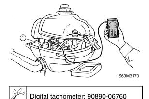
Start the engine, and then check the engine idle speed. Adjust if out of specification.
