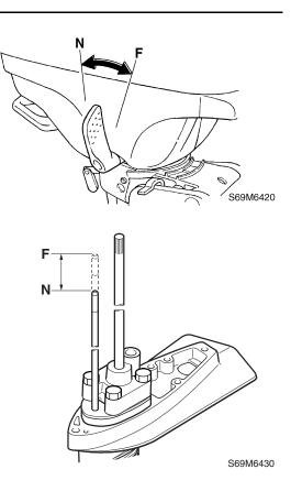
2. Install the lower unit to the upper case.
