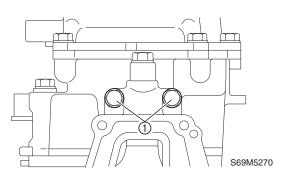
3. Remove the cylinder head bolts in the sequence shown.
