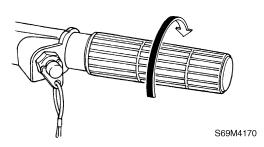
2. Make the inner wire ① of the throttle cable taut, and then connect the throttle link 2.
