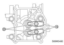
13. Install the crankcase to the cylinder block, and then tighten the crankcase bolts to the specified torques in two stage and in the sequence shown.
