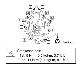
14. Install the new gasket and cylinder head cover, and then tighten the bolts to the specified torgues in two stages and in the sequence shown.
