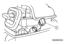
2. Place a drain pan under the drain hole, and then remove the drain bolt (2) and let the oil drain completely.
