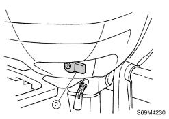
3. Place a drain pan under the drain hose, and then loosen the drain screw and let the fuel drain completely.
