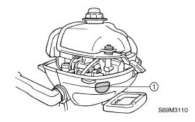
2. Disconnect the spark plug cap from the spark plug, and then remove the spark plug.
