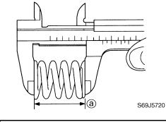
Valve spring free length (a): 35.0 mm (1.378 in) 2. Measure the valve spring tilt (b). Replace if out of specification.
