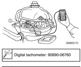
Engine idle speed: 1,800–2,000 r/min Turn the throttle stop screw ② in direction ③ or ⑤ until the specified engine idle speed is obtained.
