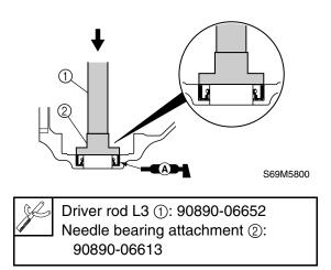
2. Install the new ball bearing into the cylinder block.
