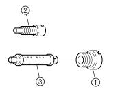
4. Check the pilot screw and needle valve for bends or wear. Replace if necessary.
