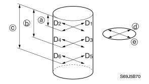
Cylinder bore (D<sub>1</sub>, D<sub>2</sub>, D<sub>3</sub>, D<sub>4</sub>, D<sub>5</sub>, D<sub>6</sub>): 54.000–54.015 mm (2.1260–2.1266 in)
